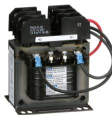
Industrial control transformer, Type TF, 1 phase, 100VA, 208V primary, 120V secondary, 50/60Hz
