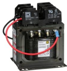
Industrial control transformer, Type TF, 1 phase, 150VA, 208/230/460V primary, 115V secondary, 50/60Hz
