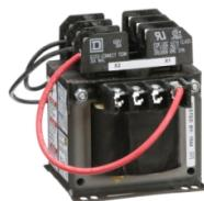
Industrial control transformer, Type TF, 1 phase, 250VA, 208V primary, 120V secondary, 50/60Hz
