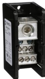
Power distribution block, Linergy, 1 pole, 1 line, 6 load, 335A Cu, 270A Al, 600V
