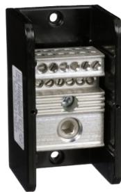
**Power distribution block, Linergy, 1 pole, 1 line, 12 load, 380A Cu, 310A Al, 600V**
