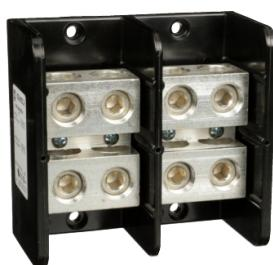
Power distribution block, Linergy, 2 pole, 2 line, 2 load, 760A Cu, 620A Al, 600V
