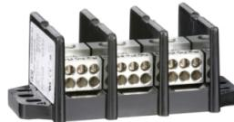
Power distribution block, Linergy, 3 pole, 1 line, 6 load, 175A Cu, 135A Al, 600V
