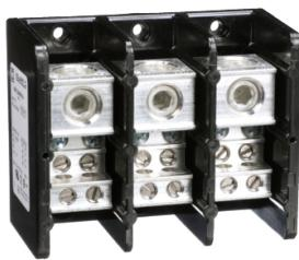
Power distribution block, Linergy, 3 pole, 1 line, 4 load, 335A Cu, 270A Al, 600V
