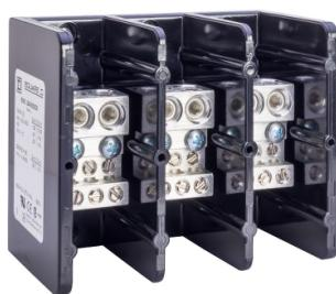
Power distribution block, Linergy, 3 pole, 2 line, 6 load, 350A Cu, 270A Al, 600V
