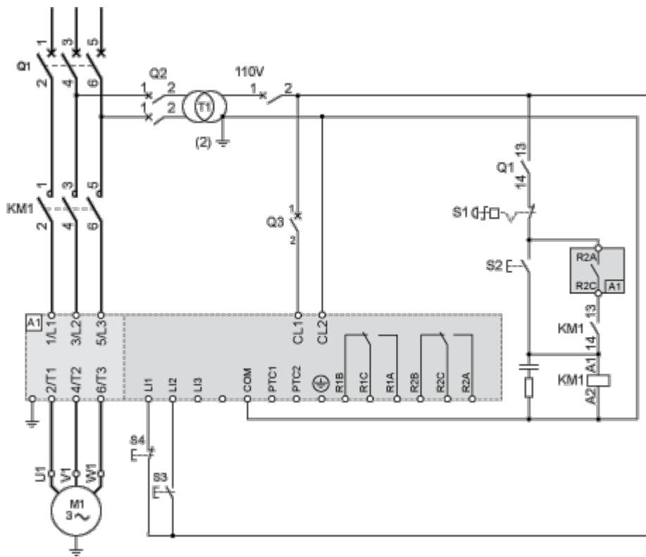
110 Vac control, Logic Inputs (LI) 110 Vac, 2-wire control, freewheelstop
