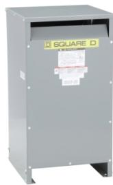
Transformer, dry type, DOE 2016, 37.5kVA, 1 phase, 600V primary, 120/240V secondary, 18H, 150C rise
