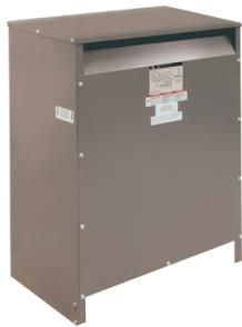
Transformer, dry type, DOE 2016, 75kVA, 1 phase, 600V primary, 120/240V secondary, 21D, 150C rise,
