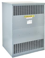
Transformer, dry type, DOE 2016, 500kVA, 3 phase, 480V delta primary, 208Y/120V secondary, 30J, 150C rise
