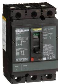
Circuit breaker, PowerPact H, 100A, 3 pole, 600VAC, 18kA, lugs, thermal magnetic, 100%
