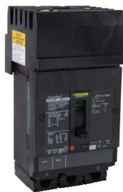
Circuit breaker, PowerPact H, 30A, 2 pole, 600VAC, 25kA, I-Line, thermal magnetic, 80%, AC
