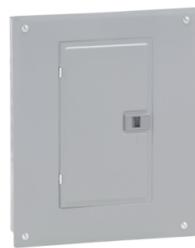
Load center, Homeline, 1 phase, 12 spaces, 24 circuits, 100A convertible main breaker, PoN, NEMA1, combo cover
