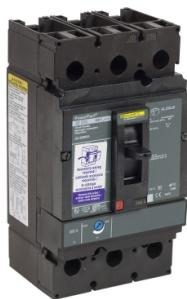
Circuit breaker, PowerPact J, 225A, 3 pole, 600VAC, 14kA, lugs, thermal magnetic, 80%, shunt
