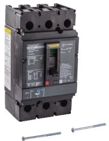
Circuit breaker, PowerPact J, 225A, 3 pole, 600VAC, 18kA, lugs, thermal magnetic, 100%
