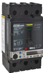
Circuit breaker, PowerPacT J, 250A, 3 pole, 600VAC, 25kA, lugs, Micrologic 6.2A, 80%
