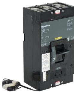
Circuit breaker, LA, 350A, 3 pole, 600VAC, 22kA, 250VDC, 10kA, lugs, thermal magnetic, shunt trip
