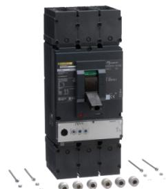
Circuit breaker, PowerPact L, 600A, 3 pole, 600VAC, 18kA, lugs, MicroLogic 3.3, 80%
