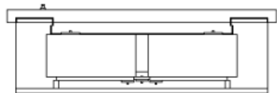
Typical Mounting of QO/QOB Circuit Breakers
