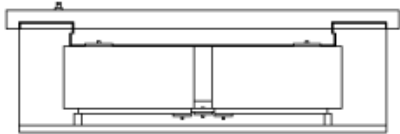
Typical Mounting of QO/QOB Circuit Breakers
