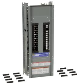
Panelboard interior, NQ, main lugs, 100A, Cu bus, 30 pole spaces, 1 phase, 3 wire, 240VAC, 48VDC, 14in W
