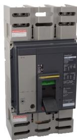
Circuit breaker, PowerPact P, 1200A, 3 pole, 600VAC, 18kA, lugs, Micrologic 3.0, 100%
