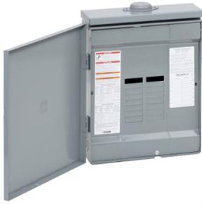
Load center, QO, 1 phase, 12 spaces, 24 circuits, 125A convertible main lugs, PoN, NEMA3R, gnd bar
