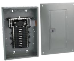
Load center, QO, 1 phase, 24 spaces, 34 circuits, 125A convertible main lugs, PoN, NEMA1, gnd bar, combo cover
