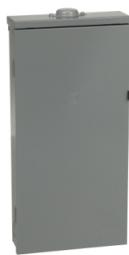
Load center, QO, 1 phase, 30 spaces, 30 circuits, 200A convertible main lugs, PoN, NEMA3R, gnd bar
