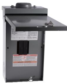
Load center, QO, 3 phase, 3 spaces, 3 circuits, 60A main lugs, NEMA3R, neutral gnd bar
