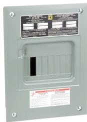
Load center, QO, 1 phase, 8 spaces, 16 circuits, 100A fixed main lugs, NEMA1, flush cover
