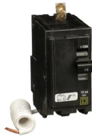
Mini circuit breaker, QO, 15A, 2 pole, 120VAC, 10kA, bolt on, switch neutral
