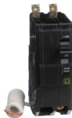
Mini circuit breaker, QO, 20A, 2 pole, 120/240VAC, 10kA, bolt on, 30mA grd fault B [TAA]
