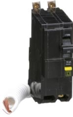
Mini circuit breaker, QO, 30A, 2 pole, 120/240VAC, 10kA, bolt on, 6mA grd fault A, pigtail [TAA]
