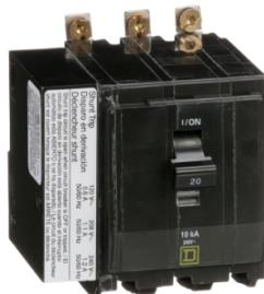
Mini circuit breaker, QO, 20A, 3 pole, 120/240VAC, 10kA, bolt on, AC shunt
