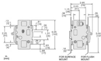
2.50 [64] MIN. WIRE BENDING SPACE FOR 2 AWG
