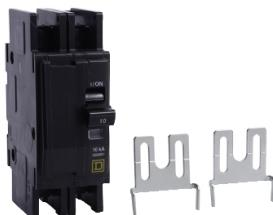
Mini circuit breaker, QOU, 20A, 2 pole, 120/240 VAC, 10kA, field reversible lugs, ring terminal, China certified
