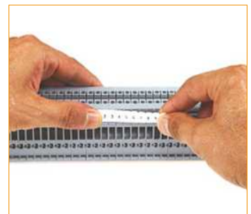
Quick labelling thanks to strips
