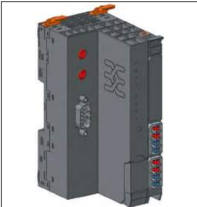
Fieldbus coupler UR20-FBC-CAN (Order No. 1334890000)
