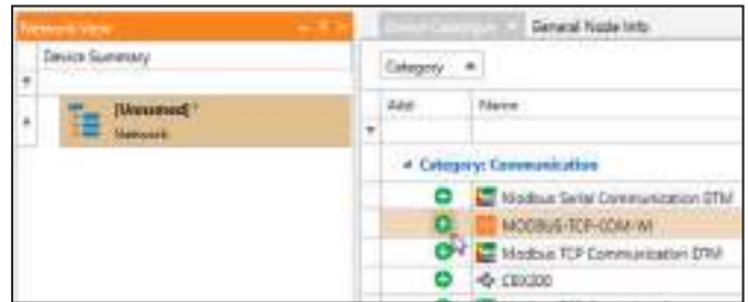
Adding the MODBUS-TCP-COM-WI DTM to the network view
