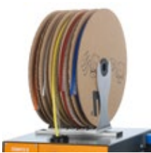
Processing of linked, reeled wire-end ferrules
