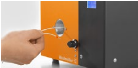
Stripping and crimping in one step
