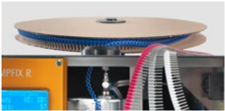
Automatic cross-section adjustment from 0.5 to 2.5 mm²
