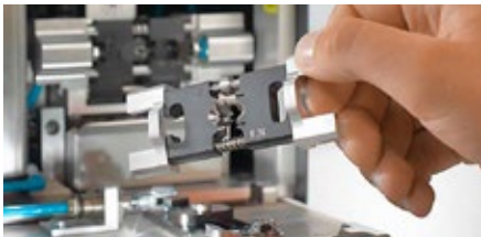
Quick-change tool for extremely short retooling times
