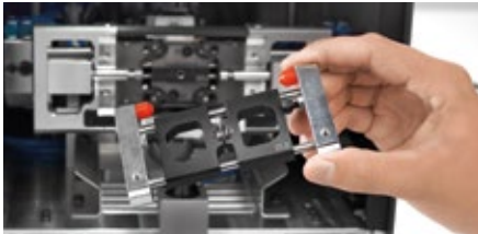
Quick-change tool for extremely short retooling times
