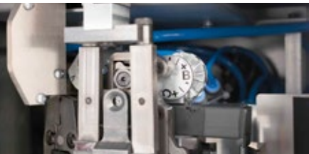
Adjustable trigger sensor for optimum stripping length
