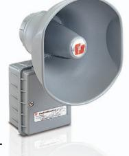
The Federal Signal Model AM15 is a rugged, re-entrant speaker for use in public address or paging applications. This 15 watt speaker features a rugged speaker cone and projector constructed of spun aluminum. The speaker wiring connections are enclosed in a dust- and moisture-proof, die-cast aluminum compartment. All external surfaces are sealed with gray powder coat paint.
