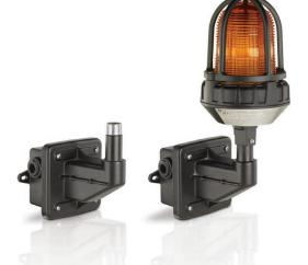
Federal Signal's Model LHWB Hazardous Location mounting bracket is specifically designed for use with Federal Signal's stationary warning lights to provide an easy and consistent means of securely mounting lights throughout a facility. The bracket features a 3/4-inch NPT male pipe connection. Optional bushings are available for 1/2-inch and 1 inch fixture mounting.
